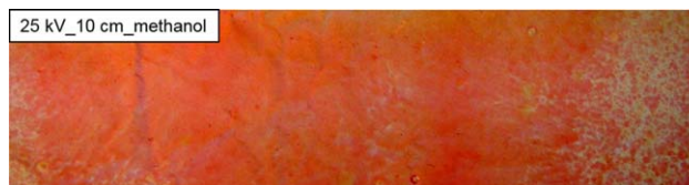
Figure 4. Initial characterization of electro spray method. Photograph of solvent dispersion on Nylon 6 membranes with multi-jet spraying set-up. The drum collector was stationary and electro spraying occurred for 10 s. [Color figure can be viewed in the online issue, which is available at wileyonlinelibrary.com .]
